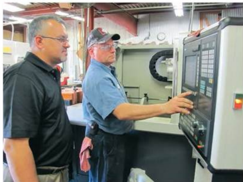
Shop owner Chris Klanica (left) and machinist Tim Wolf review programs for jobs scheduled to run on the deep-hole machine. The Siemens 828D control enables shopfloor programming of three-axis work, including automated routines for bolt hole circles and other patterns.
