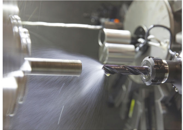
Acoustech Systems' NRT module drills stainless steel.
