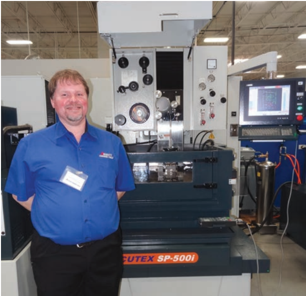
(left) Mike Kraft, EDM Applications Engineer, with the AccuteX EDM SP-500i. The SP-500i has travels of 19.7" X, 11.8" Y and 11.8" Z and 3.90" x 3.90" for the UV axis. Maximum workpiece size is 38.4" X, 22.6" Y and 11.6" Z with a workpiece capacity of 3,400 lb. It features Auto Wire Threading (AWT), this includes an AWT Skip Function and AWT Monitor Screen on the 64-bit Windows CE Control. (top right) Absolute Machine features AccuWire, its own brand of EDM Wire.
