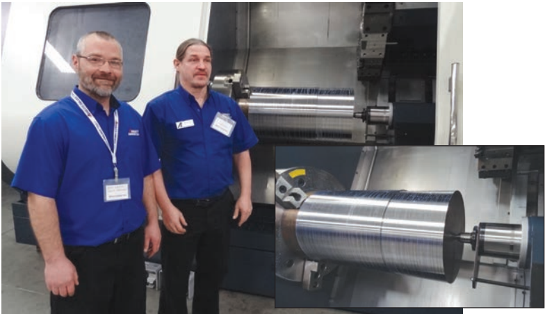
(l-r) Nate Walker, Service Manger, and Lee Soukup, Applications Engineer, Absolute Machine Tools, with the Johnford Super Turning ST-60CH performing a large shaft demo. It features a one-piece 60° cast iron bed with 39.4" swing over bed and 31.5" swing over the cross slide.
