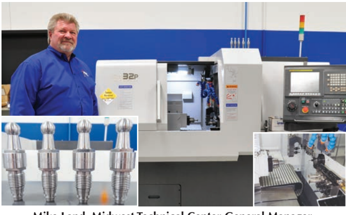
Mike Land, Midwest Technical Center General Manager, Absolute Machine Tools, with the Nexturn SA-32P 7-Axis Swiss-Type Turning Center with 32 mm capacity and 210 mm length equipped with a 12' Bar Feeder. Demo is Spherical Fitting ø1" 1144 Stressproof Bearing Steel, polished and ground.
