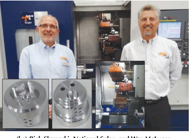
(l-r) Rick Shanoski, National Sales, and Wes McLucas, President, MD Tooling, with the Tongtai TNL-100TLSB+Y featuring a sub-spindle, live tools, bar package turning center.
