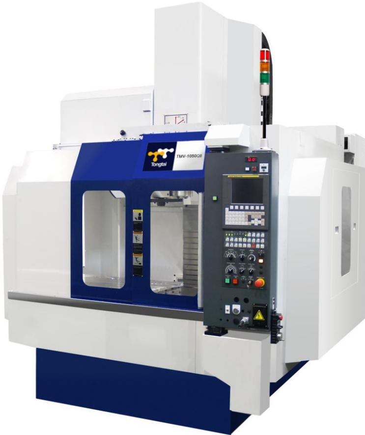
At Amerimold 2013, machine tool importer Absolute Machine Tools will exhibit the TMV-1050Q-II ultra-high performance, heavy duty vertical machining center from Tongtai Machine & Tool Co., Ltd. Well suited for both high-volume machining applications as well as mold/die work, the machine combines speed, rigidity and precision as it features a 15,000 RPM direct-drive spindle, 1,890 ipm (47,250 mm/min) rapids on all 3 axes, as well as oversized servo motors and ballscrews.
