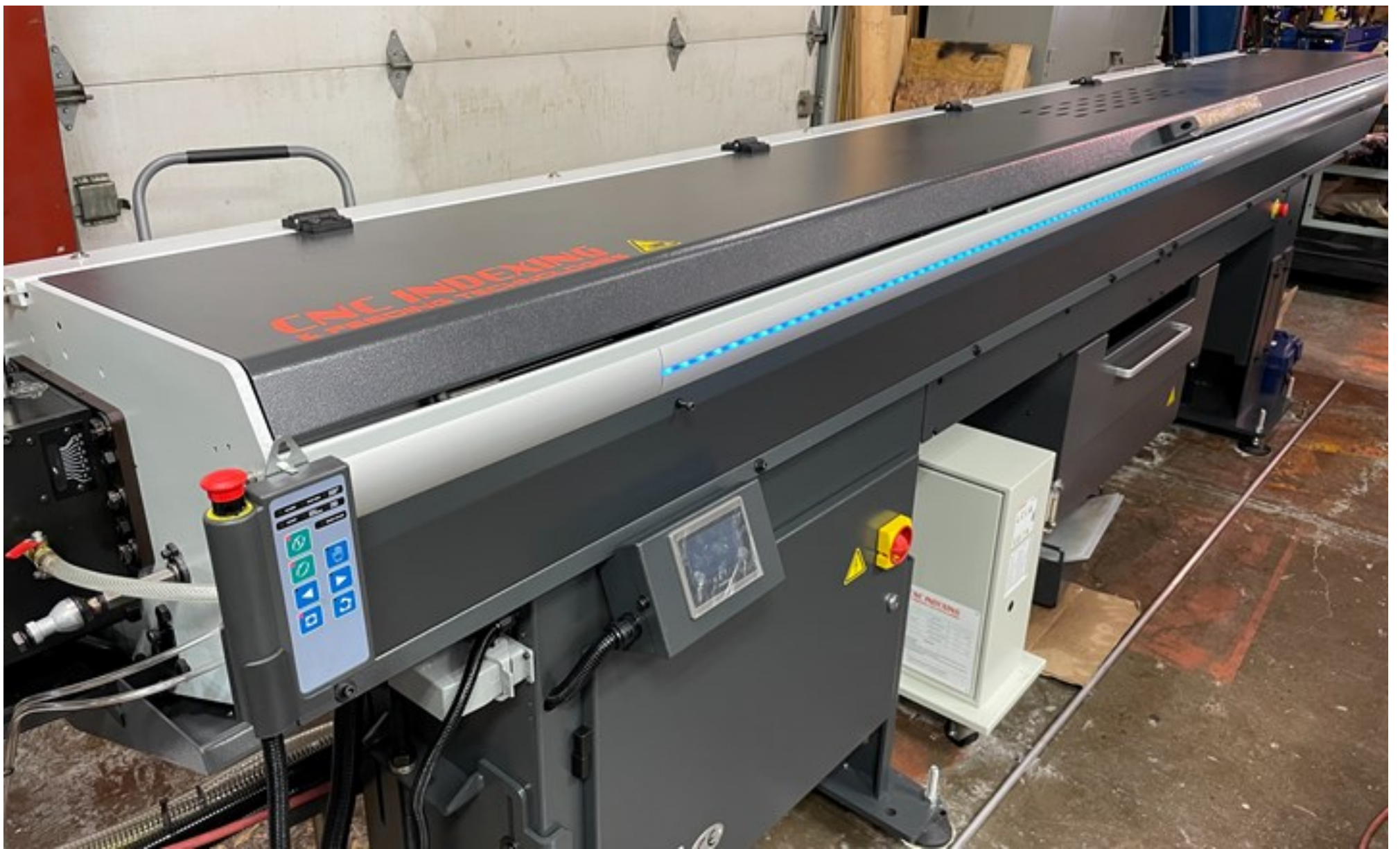
The Swiss-type's Tracer magazine bar feeder that can accommodate 12-foot-long bars includes external LED lights that offer at-a-glance visual monitoring of alarms and remaining bar length.
