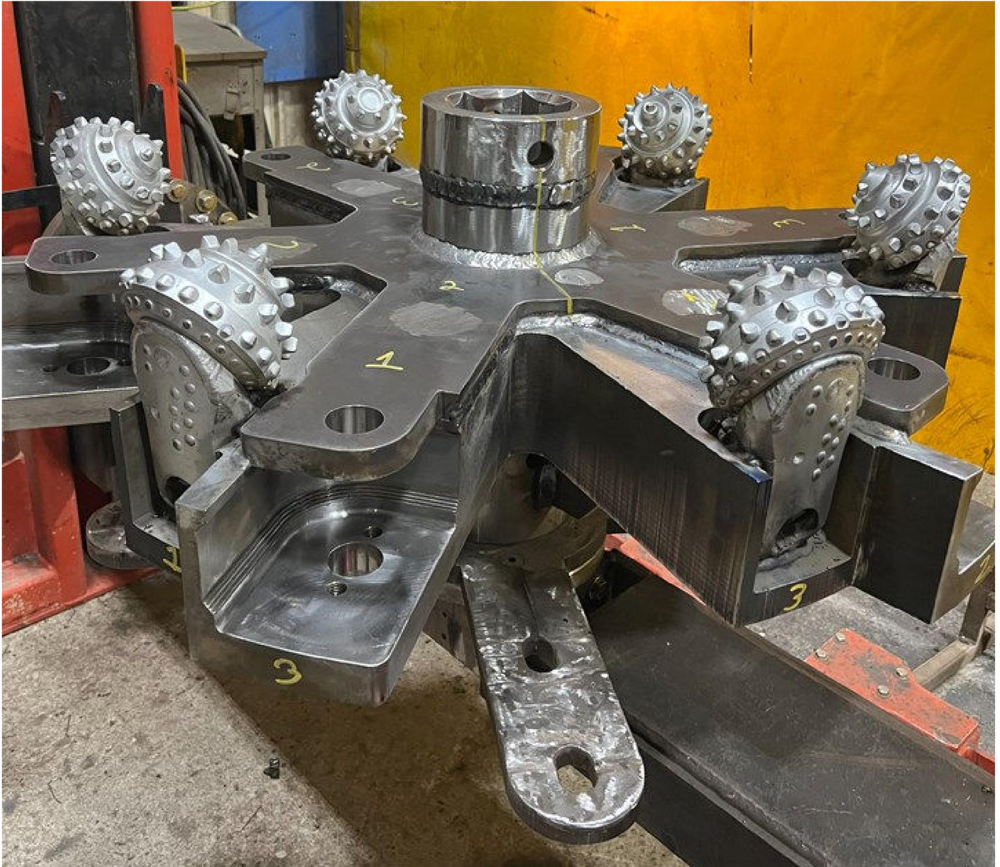
Historically, utility excavators have needed to crawl into holes to repair dull or broken drill bits. Barbco's collapsible drill head eliminates this dangerous problem for soft rock applications, as pins within the drill bits rotate to shrink the diameter of the head when the drill is put into reverse.
