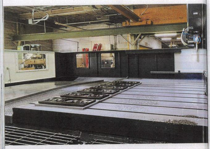
The table on the Johnford is large enough for Barbco to set up different projects on different portions of the table, using G stops to indicate which section of the table the machine should work on at a particular time. This lets the company keep parts set up if it needs to change focus for a rush order, or if one project runs into problems that can't immediately be resolved.
