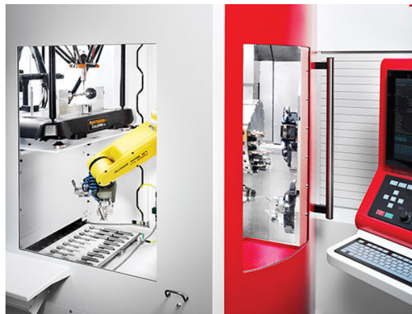
The Index iX Center automated cell is intended for lights-out manufacturing, and utilizes a pallet system for material management and a FANUC robot to pass parts to a Renishaw gauge or CMM. (Provided by Index)
