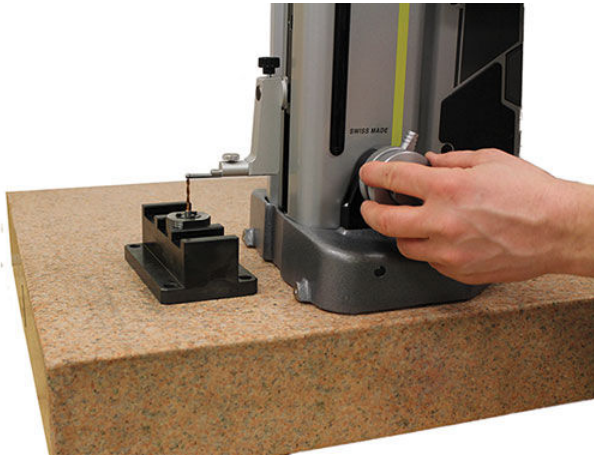
Offline measurement of cutting tools does not require any special equipment, as shown in this example using a presetting block from National Machine Products. (Provided by Tsugami/REM Sales)
