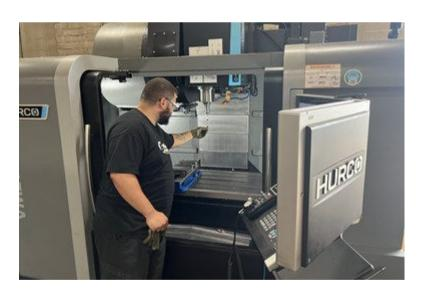
In addition to the Johnford mill, Barbco bought a Hurco VM20i three-axis mill earlier this year from Reynolds Machinery in Dayton, Ohio. With chip hopper and through-spindle coolant add-ons, the machine is fast and strong enough to match the output of the company's larger VMX 60. Now, the shop uses the Johnford for its larger parts while tasking the Hurco with smaller parts.
