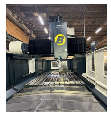
Barbco's Johnford DMC-4100PH is not the largest machine in Johnford's catalog — but it was the largest that could fit in Barbco's facility. The table can hold extremely heavy parts, supporting a total weight just over 11 tons.
