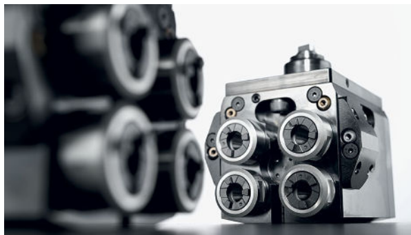
Manufacturers are increasingly asking for live tooling with their lathes that includes sensors for data monitoring, along with multiple spindles, as shown here.
