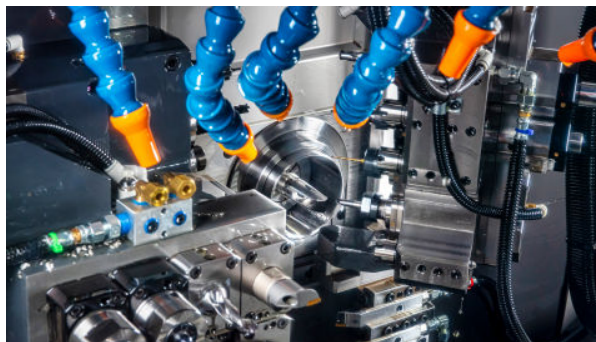
Tsugami America's SS327-III-5AX 32 mm, B-Axis Sliding Headstock Swiss Type Lathe. (Provided by Tsugami America)
