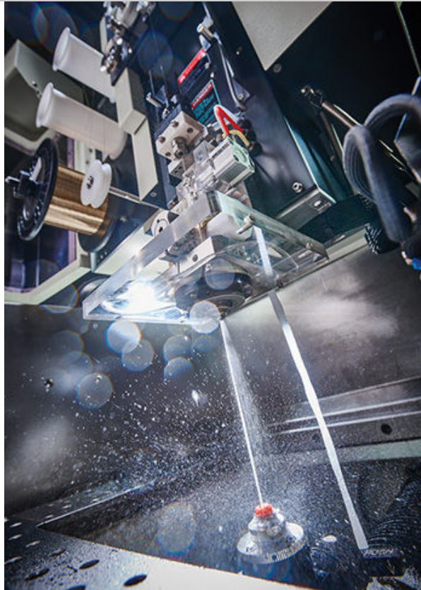
The U6 HEAT Extreme featuring coated wire technology reportedly increases rough machining rates up to 300 percent over traditional 0.010" [0.25mm] brass wire while maintaining comparable consumption rates. (Provided by Makino Inc.)
