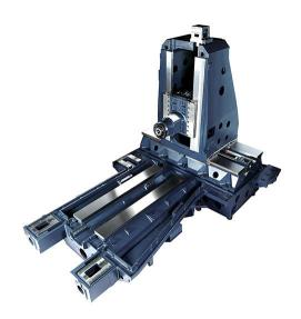
The "core" of a Doosan NHM HMC. Boxways offer superior stiffness and vibration dampening, making them popular for heavy-duty cutting, but they require more maintenance than linear guideways. (Provided by Doosan)
