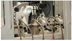
Mitsui Seiki makes its own precision thread grinders and produces its own HMC ballscrews, helping assure the longevity of these critical components. (Provided by Mitsui Seiki USA)
