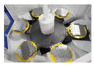
It's possible to cost-effectively add a pallet pool in the field, like this KIWA KH-4500kai pallet changer, enabling more unattended hours with a higher mix of parts. (Provided by Methods Machine Tools)
