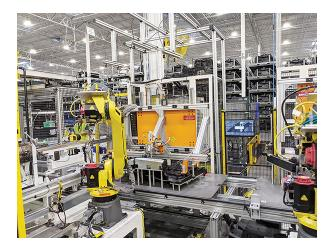
A chip assembly workcell at a Tier 1 automotive supplier that uses an Apera AI vision system to guide an industrial robot to place chips in an injection-molded subassembly. (Provided by Apera AI)
