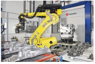
Fastems MMS for Part Handling offers batch production and setup scheduling for CNC lathes and machining centers. (Provided by Fastems)
