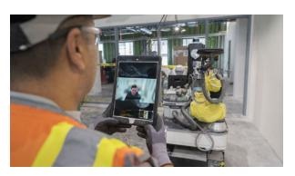
As with many robotic solutions, Canvas provides remote support to its users through a mobile device interface. (Image provided by Universal Robots USA)
