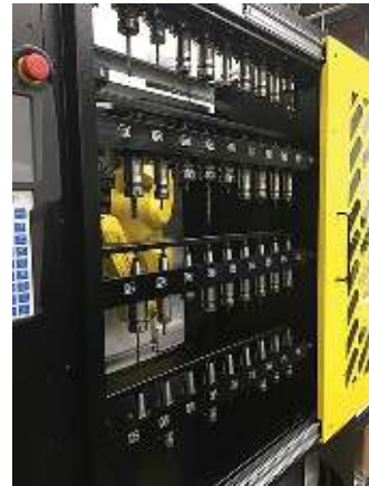
Generous tool magazines and so-called "wine racks" are essential to reducing setup time in high-mix, low-volume machining environments. (Provided by Methods Machine Tools)
