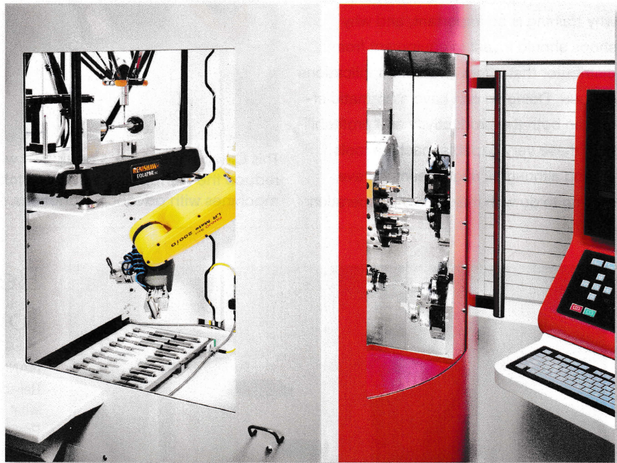
The Index iX Center automated cell is intended for lights-out manufacturing and utilizes a pallet system for material management and a FANUC robot to pass parts to a Renishaw gauge or CMM. (Provided by Index)
