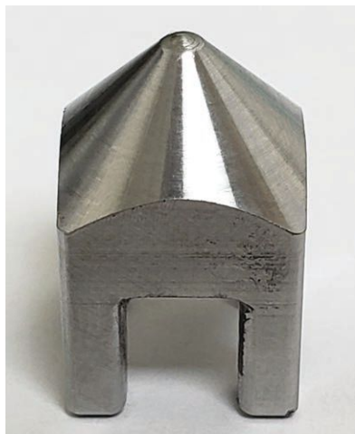
Stainless steel alloy component for an oil-field mud pump was machined using Swiss solution in Mastercam 2021 Lathe.
