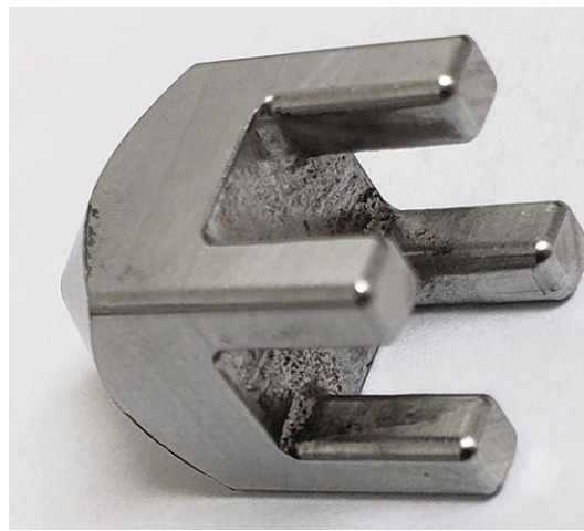
Stainless steel alloy component for an oil-field mud pump was machined using Swiss solution in Mastercam 2021 Lathe.
