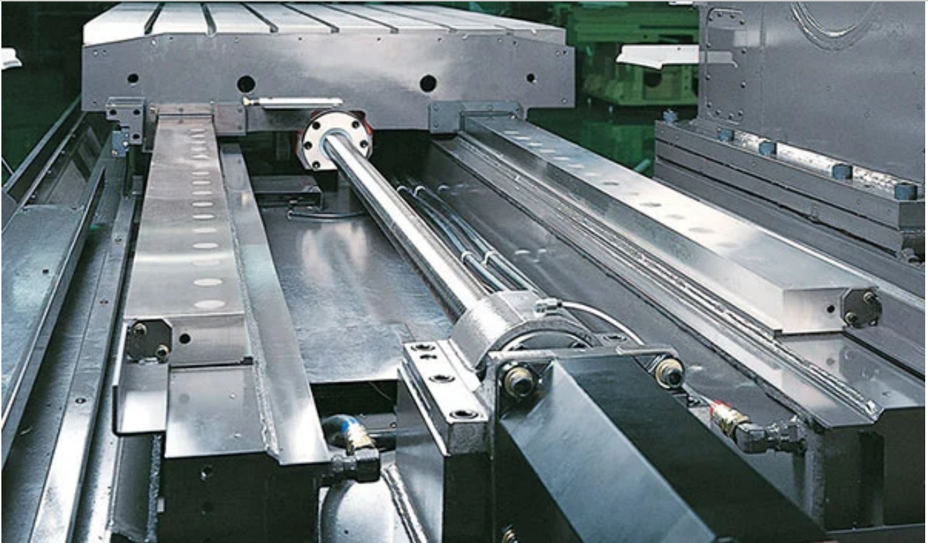
This 1218V bridge-style machining center from YASDA features precisely-ground guideways fastened to a hand-scraped mounting surface after lapping. (Provided by Methods Machine Tools)
