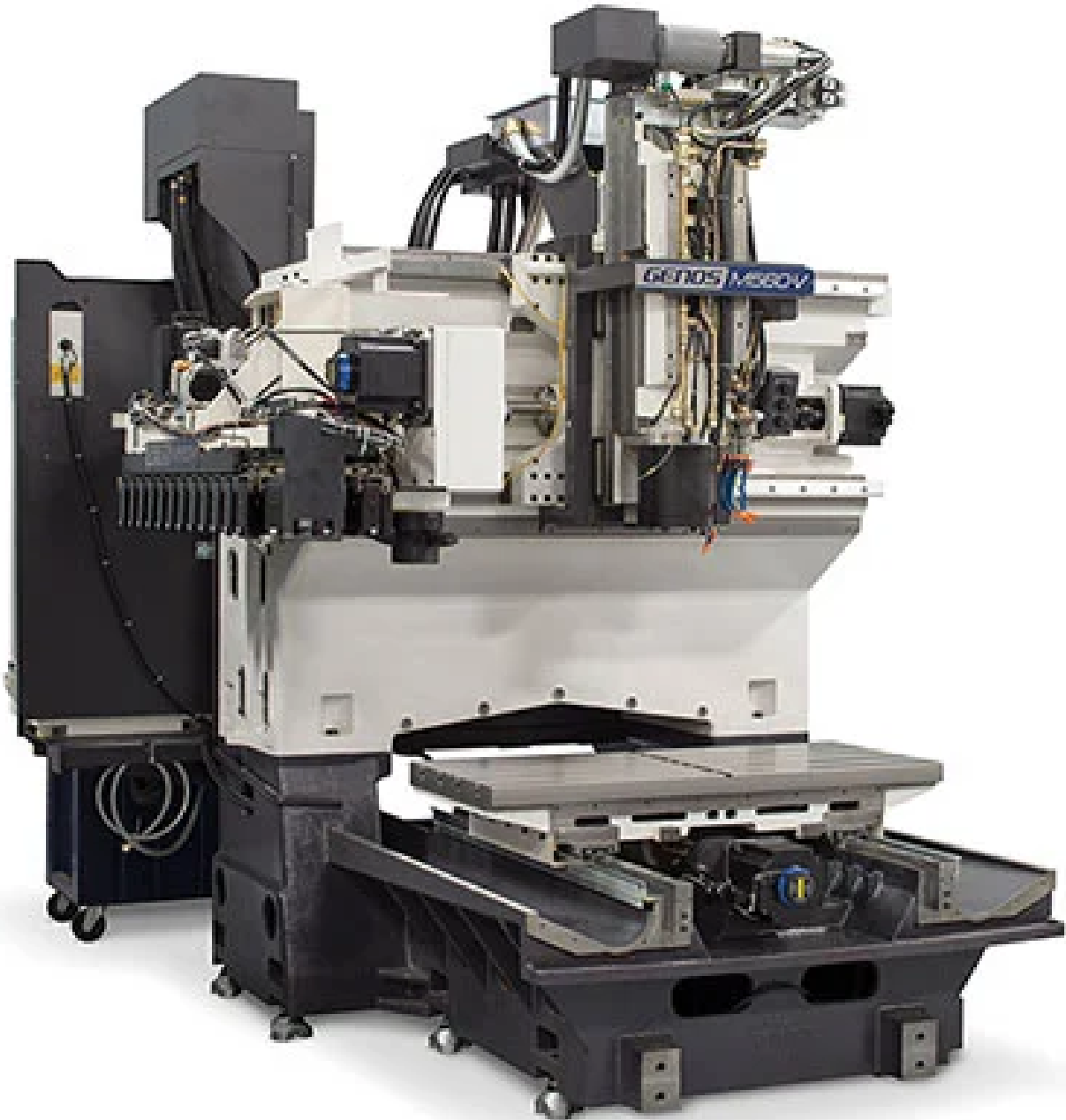
This Okuma GENOS M560V, with its sheet metal and control removed, illustrates the vertical machining center's bridge-style construction. (Provided by Okuma America)
