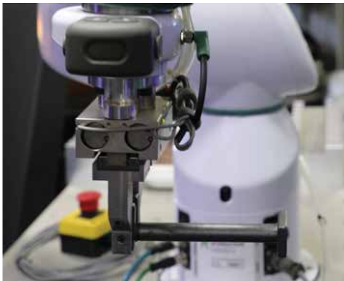
To consistently grip the silicon iron core part shown here, Absolute Machine Tools devised a pneumatic gripper for the OB7.
