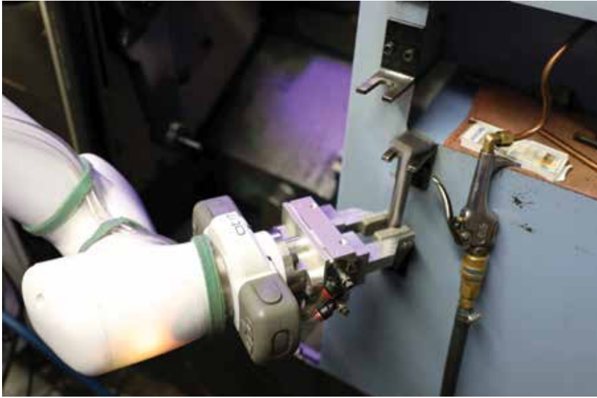
The OB7 places the part in the loading station.
