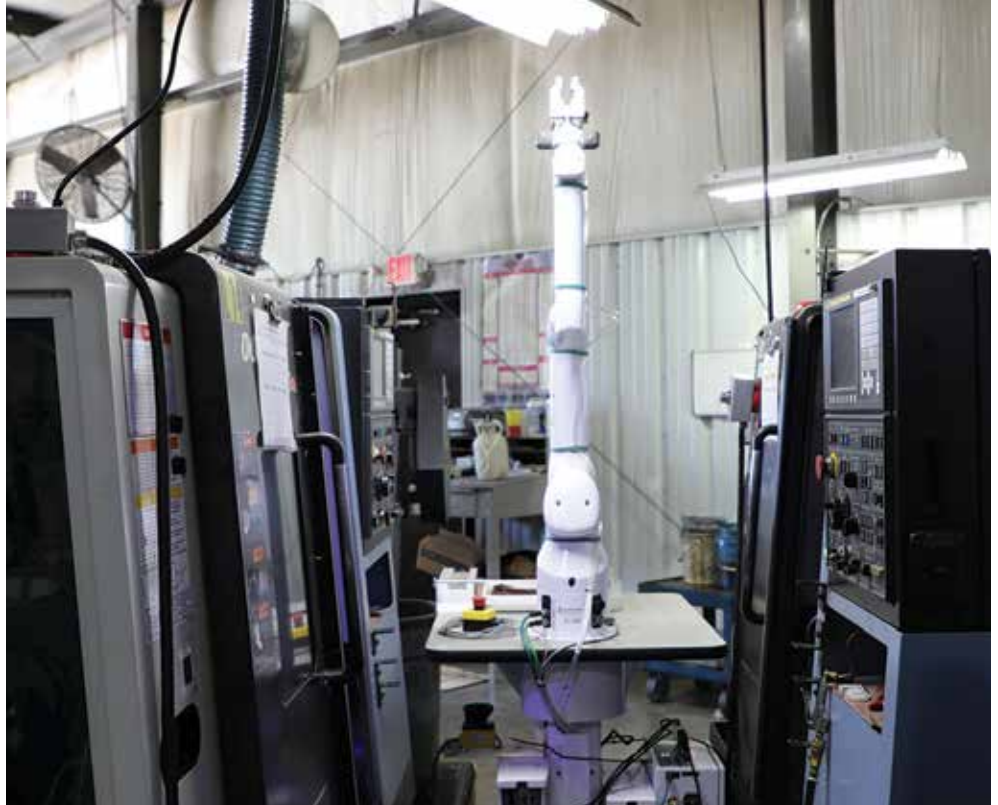
The OB7 cobot arm serves two Doosan turning machines at B.I.C. Precision Machine Co. Inc.
