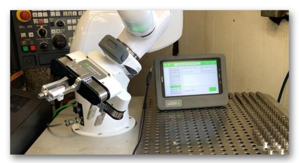
In lathe operations, which generally have short cycle times requiring an operator to constantly wait for the machine, using a dual gripper frees up time and allows the operator to focus on preparing other jobs and parts.
