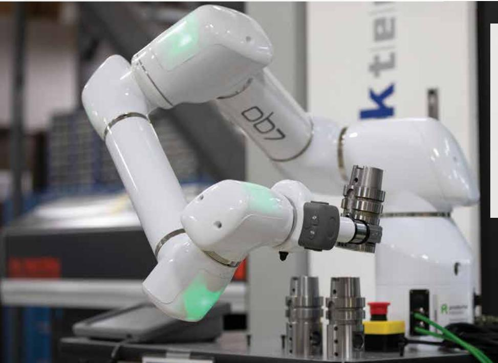
There are several collaborative robots out there, but OB7's 7 axes allow us to place the robot next to the machine door rather than in front of it, freeing up space for our machine operators. The ease of setting up OB7 has also made us profitable in our job shop environment from day one.
