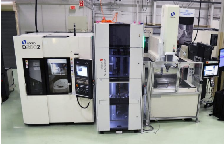
Makino’s DM automation cell can exchange both electrodes and work pieces.
