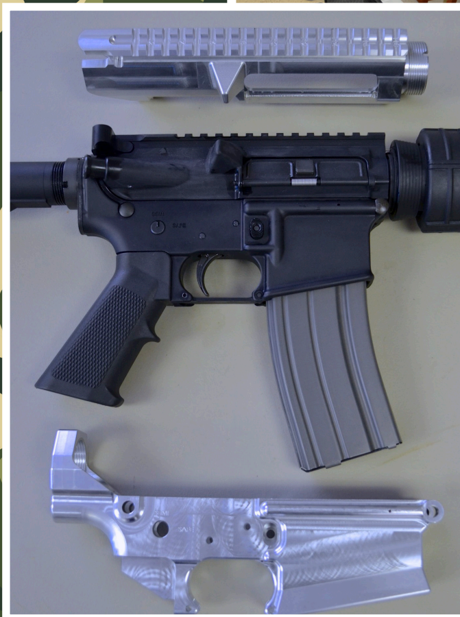
Upper and lower receivers for AR-style rifles are CNC machined from 7075 T6 aluminum forgings on a Johnford SV48 machining center.
