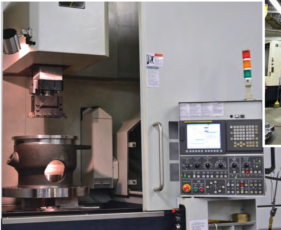
LEFT: Because the You Ji VTL 800-ATC+C is a ram-style machine, it offers a clear view of possible tool interferences during programming of machining operations. ABOVE: At 31,000 lb and with a 100" x 136" x 160" footprint, the You Ji VTL 800-ATC+C represents a solid platform for machining energy-related components at Davan Manufacturing.
