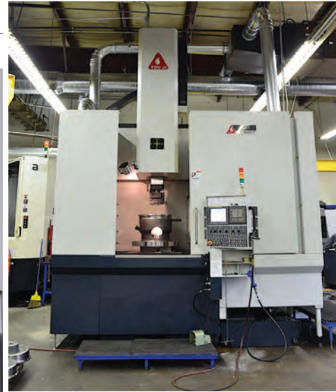
LEFT: Because the You Ji VTL 800-ATC+C is a ram-style machine, it offers a clear view of possible tool interferences during programming of machining operations. ABOVE: At 31,000 lb and with a 100" x 136" x 160" footprint, the You Ji VTL 800-ATC+C represents a solid platform for machining energy-related components at Davan Manufacturing.
